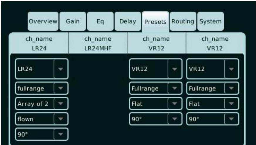
Fig 16. Bi-amp preset channel 1 disabling active control channel 2
