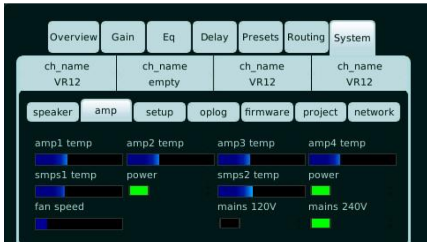
Fig 22. Amplifier status, temperature scales, fan speed level 1, AC mains 240V indication
